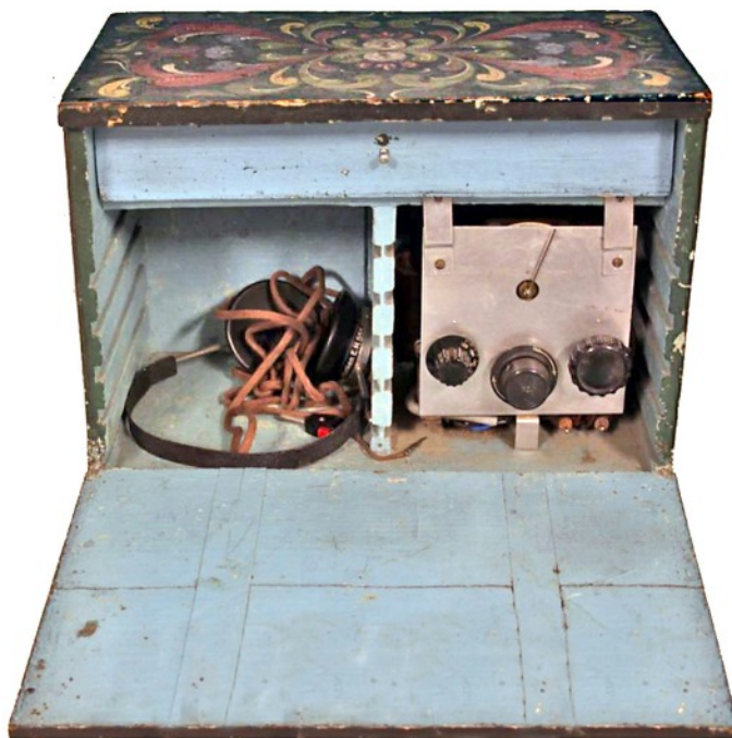
General view of an illegal homemade broadcast receiver concealed in the right hand compartment of a decoratively painted wooden cabinet. (SARK.0068)
